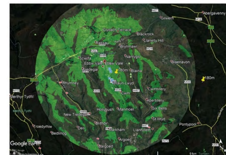
Figure B 10km Viewshed from large turbine on upland valley side above Festival Drive (450m AOD)
