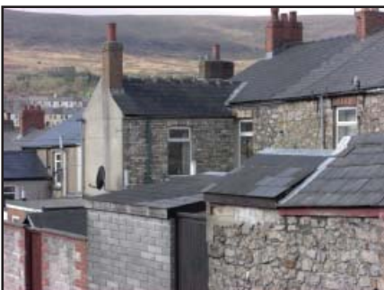
Rear extensions with pitched roofs and in materials that match the main structure are much better integrated than those with flat roofs.
