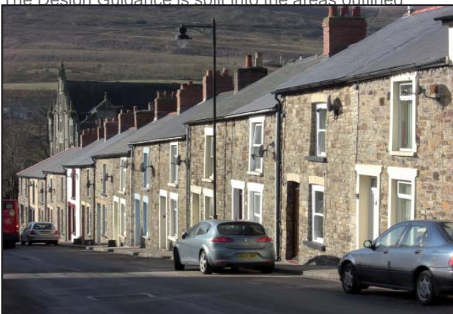
The stone-built terraces that were built in the mid 19th century have a uniformity and rhythm of elevational treatment that responds to the topography of the area in its stepped roofline. The orientation and layout of the streets allows long vistas to the surrounding hillsides providing both a visual and a physical linkage between built development and the landscape that encloses it.
