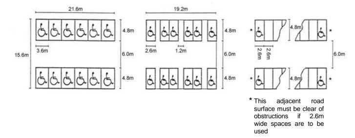
**Vehicle Bays** - The bay must be of sufficient size and be located so that the vehicle can be manoeuvred within the site, e.g. the 12m rigid lorry requires an absolute minimum of 105m² to allow it to leave a site in forward gear. Further details of good design practice can be found in appropriate Highway Authority Design Standards or 'Designing for Deliveries', Freight Transport Association 1998.
